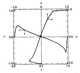
Figure 6. Velocity profiles through the centre of the cavity; Re = 10,000
