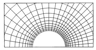
Figure 8. Mesh details near cylinder
