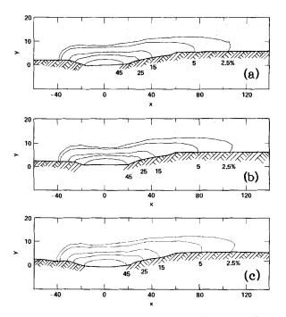
Figure 15. Predicted concentrations on a longitudinal plane: (a) 2-point, (b) mixed, (c) 1-point
