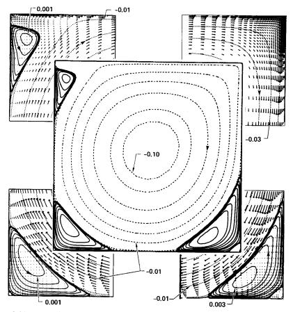
Figure 1. Flow field at Re = 5000; solid curves are  $\psi > 0$ , dashed are  $\psi < 0$ . Contours (full cavity) are: -0.10, -0.09, -0.07, -0.03, -0.01, -0.001
