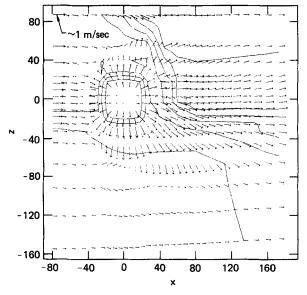
Figure 13. Horizontal velocities 1 m above the ground; 104 s after initiation of LNG spill. The spill pond is centred at (0, 0)
