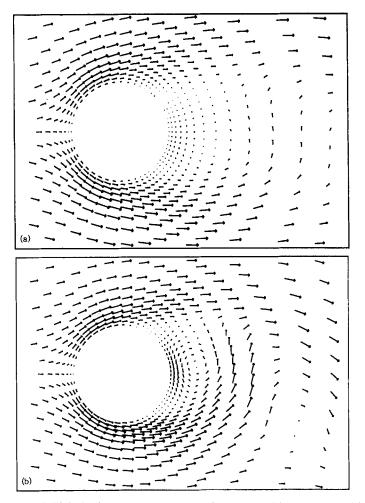
Figure 11. Velocity field near cylinder at t = 0 at Re = 50 (a) and Re = 200(b)
