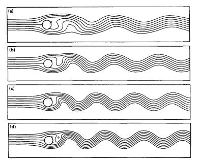
Figure 9. Streamlines during quasi-steady vortex shedding; contour values are: 0,  $\pm 0.2$ ,  $\pm 0.4$ ,  $\pm 0.6$ . (a) Re = 50; (b) Re = 100; (c) Re = 200; (d) Re = 400
