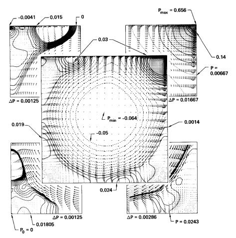
Figure 4. Same as Figure 3 except Re = 10,000 and contours (full cavity) are: -0.05 (0.00571) 0.03
