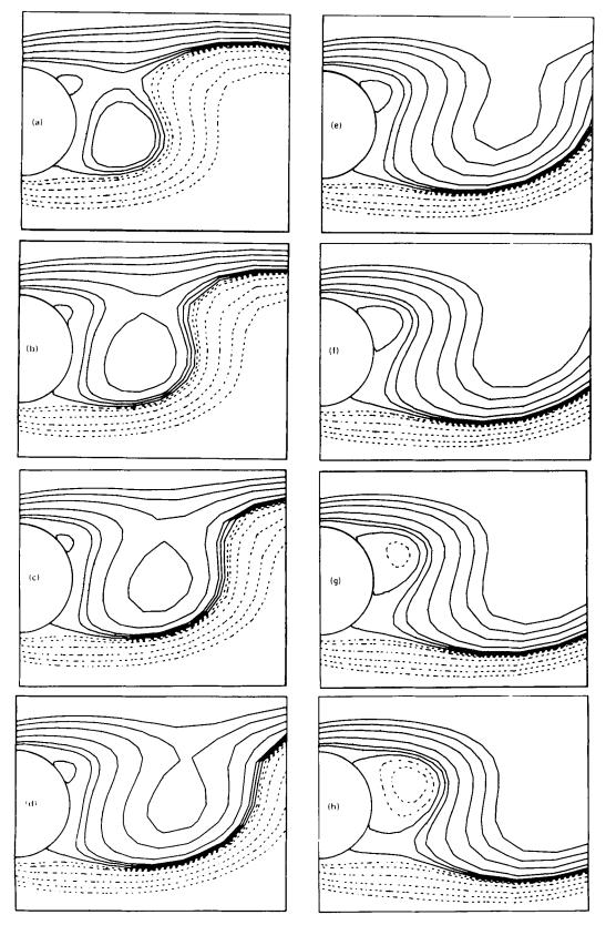
Figure 10. Streamlines near cylinder; Re = 50. Contours are:  $0, \pm 0.01, \pm 0.02, \pm 0.05, \pm 0.10, \pm 0.20$ ; solid curves are  $\psi > 0$  and dashed curves are  $\psi < 0$ .  $\Delta t = \tau/16$  between successive pictures
