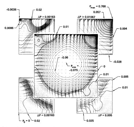
Figure 3. Isobars and velocity vectors for Re = 5000; solid curves are P > 0, dashed are P < 0. Contours (full cavity) are: -0.06 (0.005) 0.01
