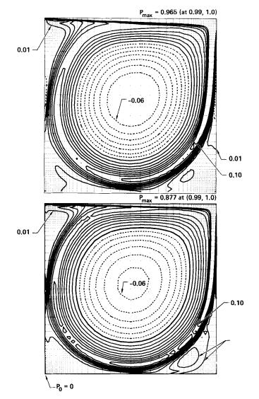
Figure 5. Total pressure fields; solid curves are  $P_T > 0$ , dashed are  $P_T < 0$ . Top: Re = 5000; bottom: Re = 10,000. Contour interval is 0.01
