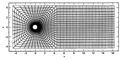
Figure 7. Finite element mesh for flow past a cylinder
